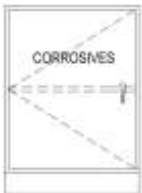
SMA24L Acid Storage Cabinet Single door left hand hinged (24" w x 35" h x 18" d)
